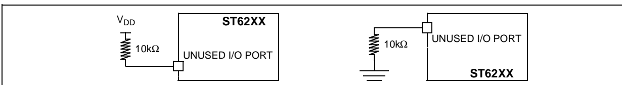
Figure 56. Two typical Applications with unused I/O Pin
